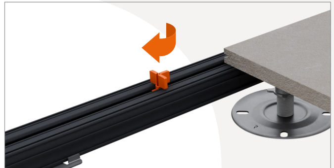
2 Insert the tile spacer into the upper groove of the joist and rotate 90 degrees.
