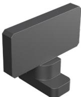
RaafT® 4mm (0.15in) 2-way spacer tabs are designed to lock into the top of a joist creating a consistent 4mm (0.15in) gap between tiles, that are loose laid onto the RaafT® system.
