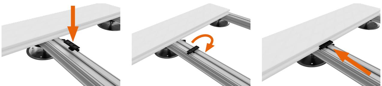
Insert the installation clips into the sub profile. Turn and push along the lower deck board edge. Clip may need to be tapped with a rubber mallet to secure firmly against the board
