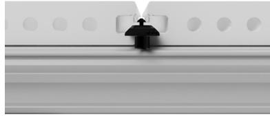
Apply the following deck boards in the same direction and an angle of approx. 15° to the installation clip and push up against the clip head. Then lower the board down and repeat across the decking area.
