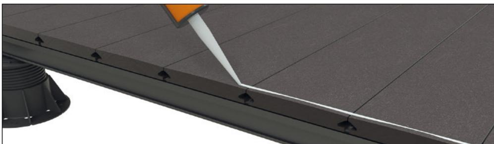
Weigh down the end profile, press on it or possibly fix it using tape, until the adhesive has set (approx. 15 min.).
